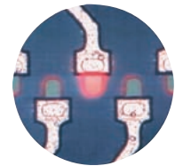
Figure 5 LED light emission Digital LEDs used in color printer. In the areas emitting red light, successive electrons and holes join up to produce light. (Enlarged 300 times).
