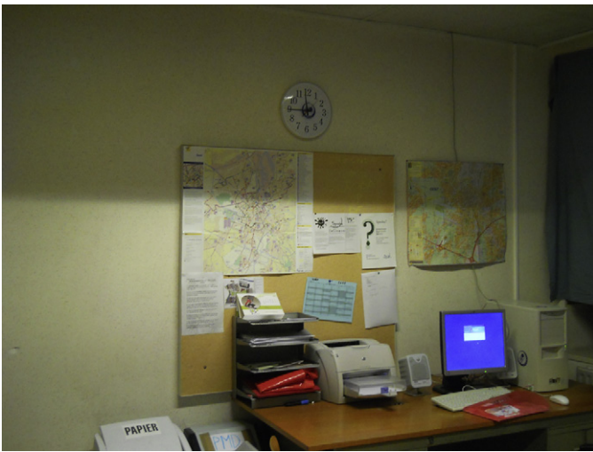
Fig. 7. Abrupt transition from dark to light on the walls (LED tube Brand I ).
