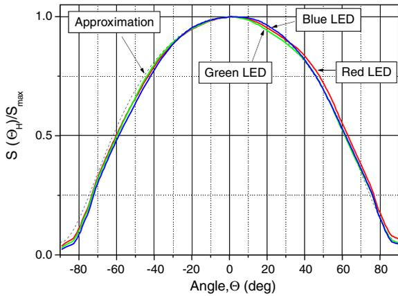
Fig. 7. Measured sensor directivity in a horizontal direction.
