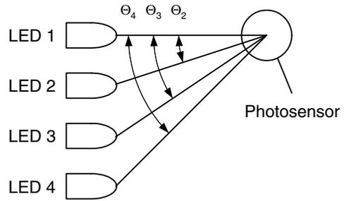
Fig. 4. Measurement system structure.
