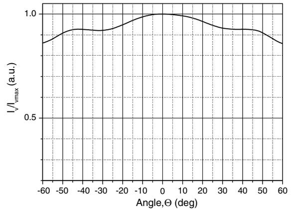
Fig. 3. Calculated screen FFP in Cartesian coordinates.
