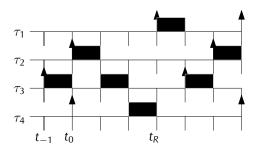
If we (artificially) redefine the release time of J<sub>i,k</sub> to be t<sub>-1</sub>, then t<sub>R</sub> remains unchanged (but the response time of J<sub>i,k</sub> may increase)
