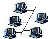
shared wire (e.g., cabled Ethernet)
