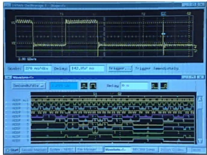
The interest of coupling the logic analyser with an oscilloscope appears on this figure. The logical analyzer provides the time of transitions, but a very coarse representation of their actual shape, which is idealized as rectangular pulses.
