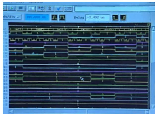
The **time analyser** looks like a digital oscilloscope with a much larger number of channels.
