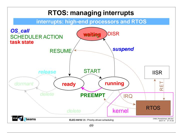
In much of modern processors, an interruption is a major event that switches in hardware the processor in a special mode/context called "kernel" or "supervisor"
