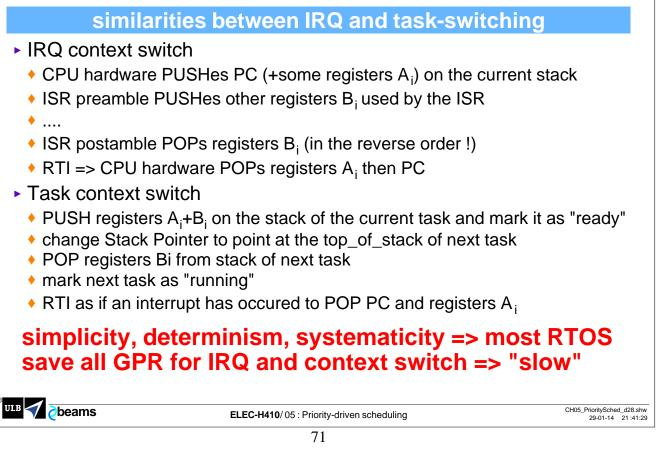
Changing the context is a mechanism which is implemented in every processor as part of the management of the interrupts. The current state of the processor (i.e. the **context**) must be saved so that the execution can resume exactly in the same condition when the interrupt has been fully serviced.
