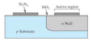
Local oxydation (make thick-field oxide appear to isolate transistors)
