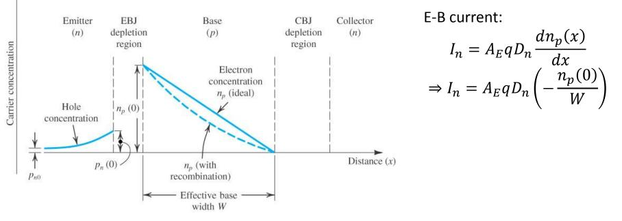
At collector side, electrons are swept through depletion region
