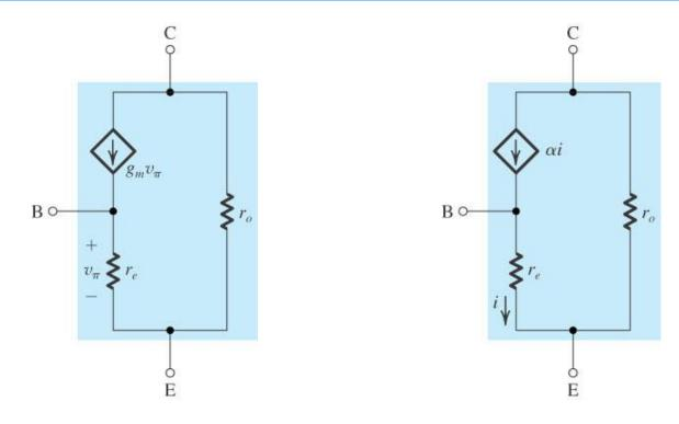
$$g_m = \frac{I_C}{V_T} \qquad r_e = \frac{V_T}{I_E} = \alpha \left(\frac{V_T}{I_C}\right) \qquad r_o = \frac{V_A}{I_C}$$
