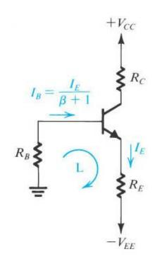
$$R_B I_B + V_{BE} + R_E I_E = V_{EE}$$
