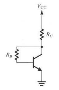
$V_{CC} = R_C I_C + R_B I_B + V_{BE}$  $V_{CC} = R_C I_C + R_B \frac{I_E}{\beta + 1} + V_{BE}$  $\Rightarrow I_E = \frac{V_{CC} - V_{BE}}{R_C + \frac{R_B}{\beta + 1}}$
