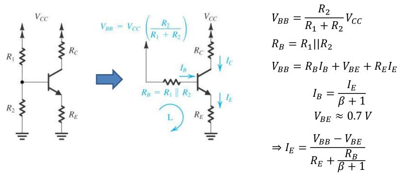
Try to make robust against transistor dispersion with  $V_{BB} \gg V_{BE}$  and  $R_E \gg \frac{R_B}{\beta+1}$
