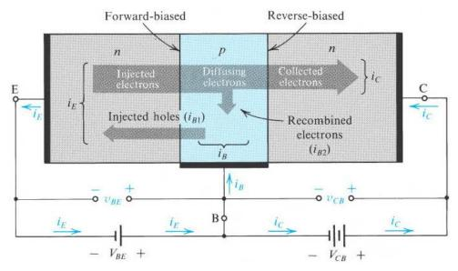
• Composed of holes injected from base to emitter
