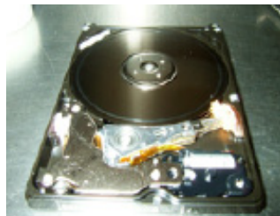
Figure 12. Head contact on platter
